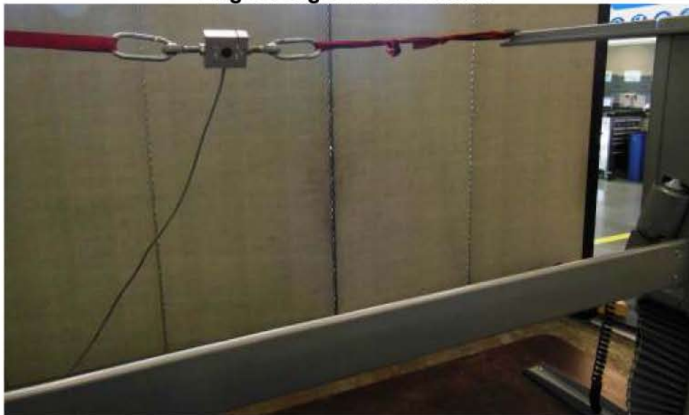
Leg Strength Test-Inward
