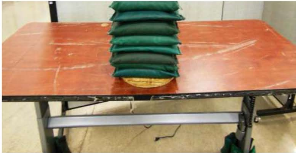
Functional Concentrated Load
